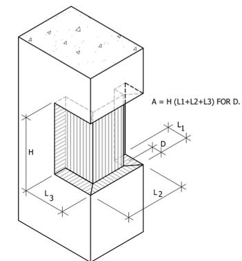
**D** MEASUREMENT PROCEDURES FOR BEAMS AND COLUMNS
