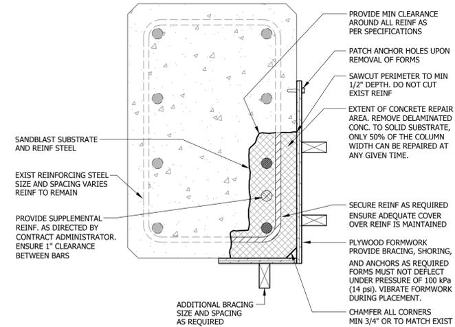
**B** TYPICAL FORM & POUR COLUMN REPAIR DETAIL
