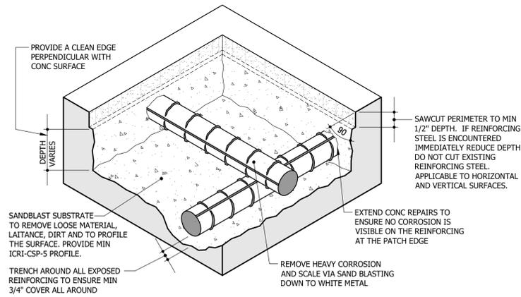
**A** TYPICAL SURFACE PREPARATION OF DELAMINATED CONCRETE
